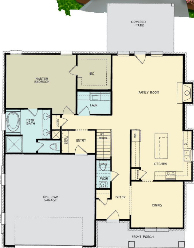
FIRST FLOOR PLAN
